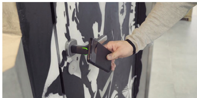
In the arena, the doors are opened with access rights stored on mobile devices and wristbands.
