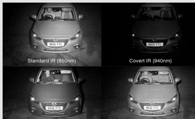
With many ANPR systems, visible light is filtered out and only IR light is used by the camera.
