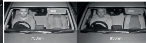
When zooming for a closer look, 730nm provided the greatest level of detail.
