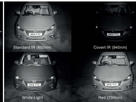
The driver recognition test revealed that three out of four wavelength examples delivered fairly good level of details inside the vehicle. However, the Covert IR (940nm) delivered significantly worse images.
