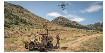
Tethered drones connect to a base station or vehicle by microfilament wire.
