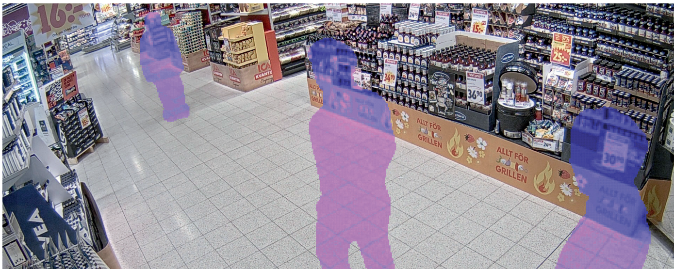
Axis Live Privacy Shield compares a live camera view to a set background scene and applies a detailed and dynamic transparent mask to areas of change.
