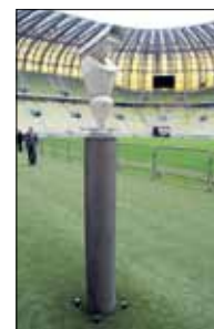
On the infield, eight cameras have been mounted on height-adjustable poles.
