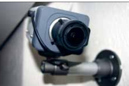
A PoE enabled IP security camera is an example of a powered device (PD) equipped to accept low voltage power transmitted over Ethernet cabling.
